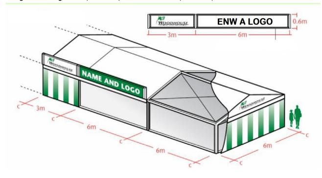
Diagram of single unit (3m x 6m) and double unit (6m x 6m):
